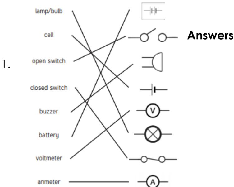
2. You should have an open switch, bulb and a battery symbol (not a cell).
